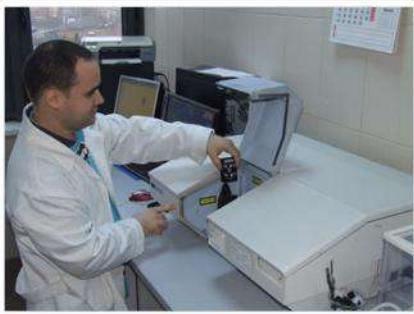
**Spectrometru FTIR Spectrum BX II Perkin Elmer**
