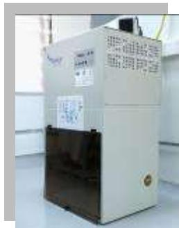
**Hota PCR (Polymerise Chain Reaction = Reactie Polimerazica in Lant) Telstar mini-V (PCR)**
