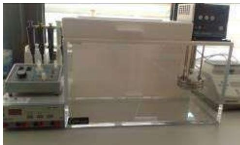
**Sistem de electroforeza DGGE model DGGEK-2001 CIPHER DGGE SYSTEM 2 PLACE**
