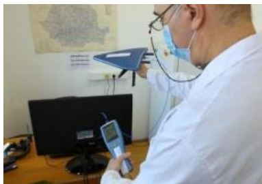
Sistem de monitorizare camp electromagnetic
